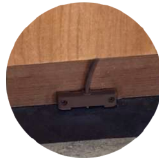
Miniature detector connected to the triangular detector and affixed to the toekick in front of the sink (available in White, Brown, Beige and Mahogany)
